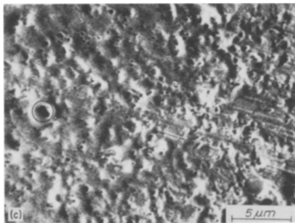
Figure 2 Surface of a ground WC-6% Co hardmetal irradiated with a Q -switched neodymium-glass laser: (a) as-received state, (b) after first laser pulse (boundary region), (c) after third laser pulse (boundary region).
