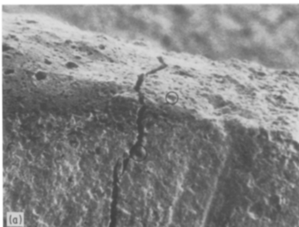
Figure 8 Side view of ground surface (bottom) with macroscopic cracks induced by unswitched laser pulses on the fracture surface of a WC-6% Co hardmetal. (a) After first laser pulse. (b) After third laser pulse; original crack has closed but opened again along a new path (see marked structural details).
