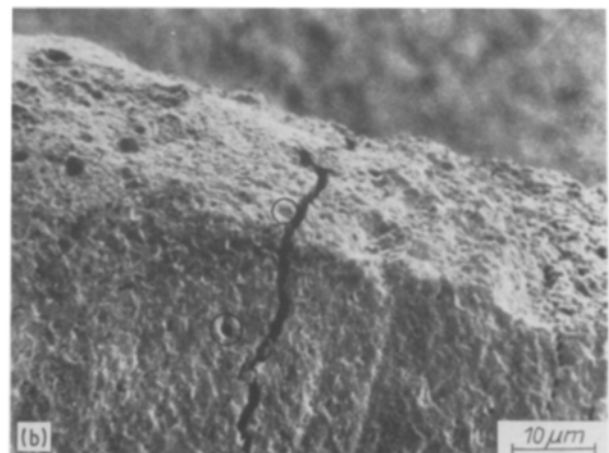
Figure 8 Side view of ground surface (bottom) with macroscopic cracks induced by unswitched laser pulses on the fracture surface of a WC-6% Co hardmetal. (a) After first laser pulse. (b) After third laser pulse; original crack has closed but opened again along a new path (see marked structural details).
