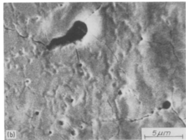
Figure 6 Surface of a polished WC-6% Co hardmetal irradiated (as in Fig. 3) with a Q-switched neodymium-glass laser. (a) After second laser pulse (boundary region); note higher energy input and local melting around large pore. (b) After twelfth laser pulse; local energy input was increased by displacing the spot centre towards the region of investigation.
